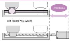
(with ball screw mechanism)
